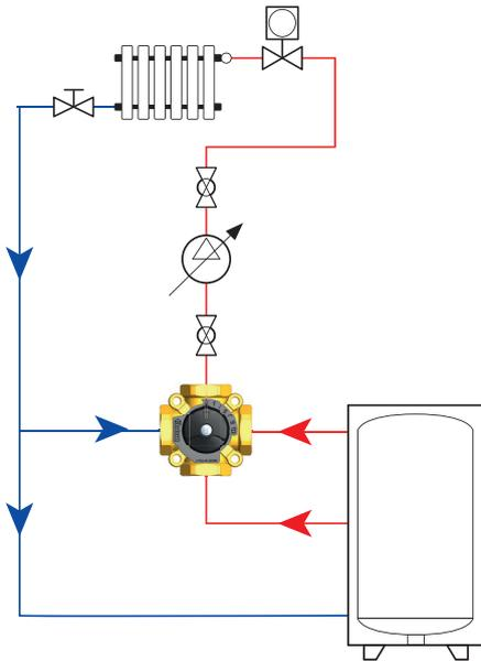
Use of V52 and V53 as diverting valves
