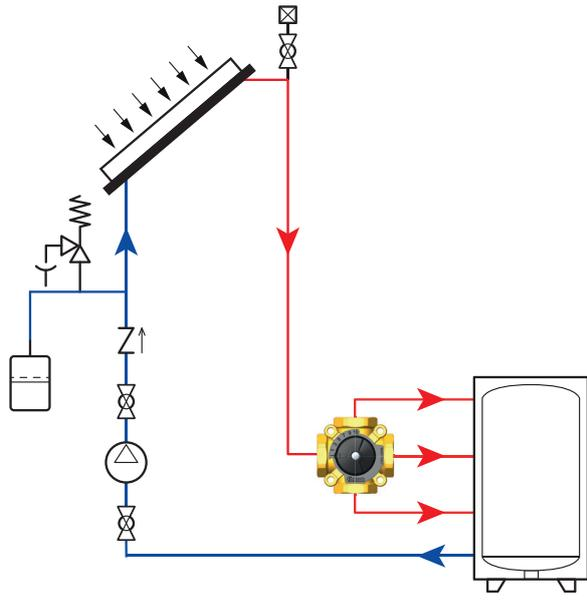
Use of V52 and V52 valves with anti-condensation function
