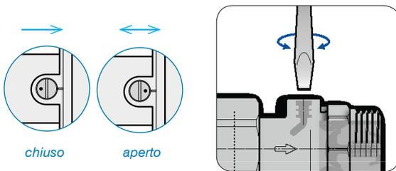
Pay attention: remember to put back into service the check valve when flushing/filling operations are completed
