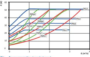
PVc: Power consumption at constant speed PDPp: Power consumption at proportional pressure PDPc: Power consumption at constant pressure
