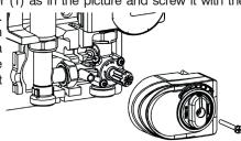
Connect the actuator to a 3 point weather compensated controller, or other device able to manage such actuator, to regu-
