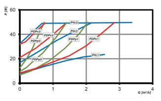
PVc: Power consumption at constant speed PDPp: Power consumption at proportional pressure PDPc: Power consumption at constant pressure rev. C
