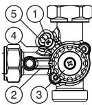
by-pass, part of the system return water is always sent to the mixed water outlet, to oblige the controller to increase the valve hot port opening. In this way, work is avoided in the vicinity of the complete closing of the hot port and the actua-
