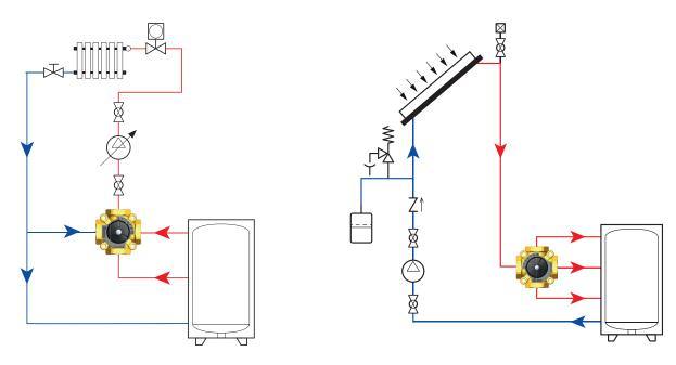
Use of V52 and V52 valves with anti-condensation function
