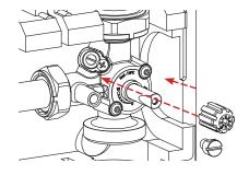
4) Rotate the valve obturator, acting on the adaptor, positioning the mark on the adaptor (3) at 45° between the hot inlet port and the system return port (corresponding to half way of the mixing valve run).
