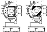
flow upward, downward or with the group laying on a side. Pay however the maximun attention to correctly fix the group to the wall when installed laying on a side.
