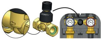
**Heat metering:** 25G.DN25 groups are equipped with specific extension to install energy metering devices, G 3/4 110 mm or G 1 130 mm. They are also complete with pocket for immersion temperature probe on the red knob monobloc.
